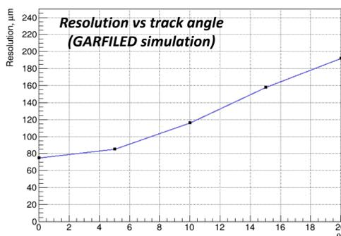
Micromegas operation in the magnetic field
