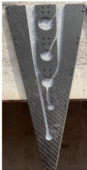
Grooved carbon fiber backplate v1 prototype
