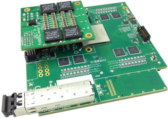
ADC64s2 (designed for MPD) is a 64-channel 12-bit 62.5 MS/s ADC with signal processing core and Ethernet interface. It has dedicated serial links for clock synchronization and data readout. *Was it tested in a trigger-less mode?*
