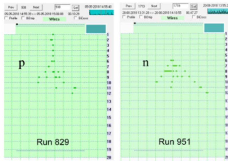
Figure 43: Demonstration of PID abilities – (a) proton vs. muon, and (b) proton vs. neutron.
