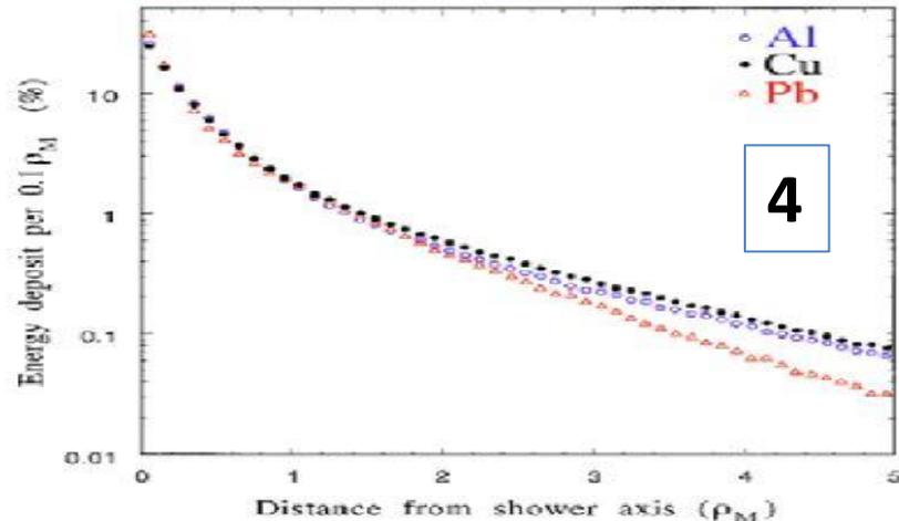
Measurement of the present electromagnetic calorimeter was fulfilled in positive beam of charged particles with an energy of  $5.0 \pm 0.2 \text{ GeV}$ . The beam size was set by a scintillation counter  $4 \times 4 \text{ cm}^2$ , installed in front of the calorimeter. The energy spectra in individual groups are shown in Fig. left. The equalization of signals was done take in account signals from  $\mu$ .
