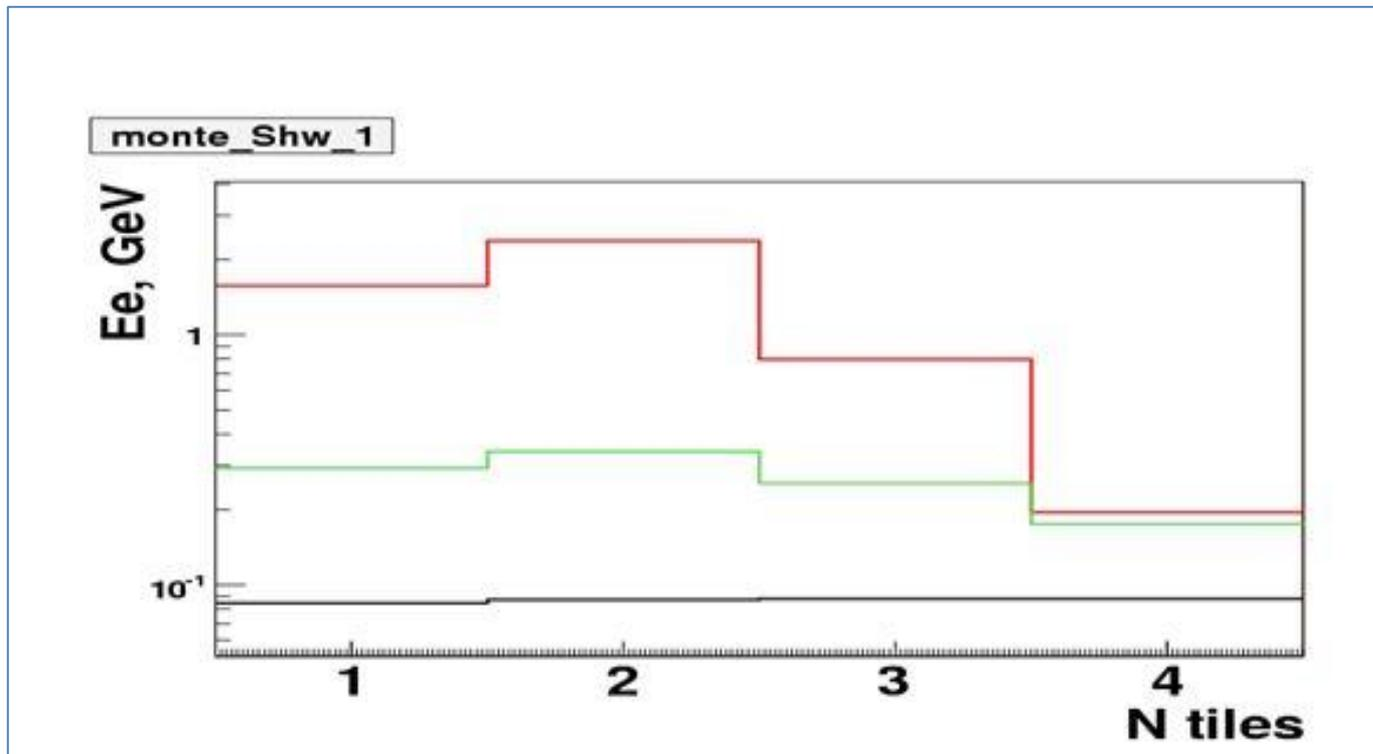
We can define the  $\chi^2$  distributions as the square deviation of the Monte Carlo values and experimental results normalized to the corresponding RMS - red lines.
