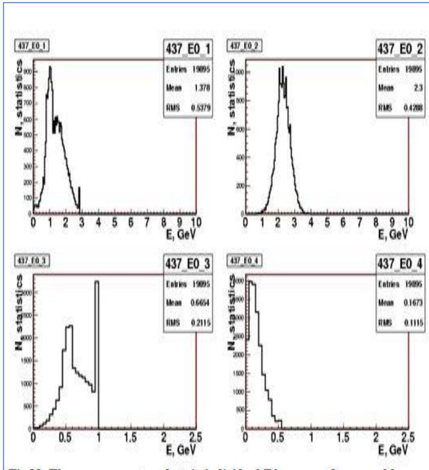
The  $e^+$  energy spectra in 4 calorimeters tiles are shown after  $\chi^2$  rejection.
