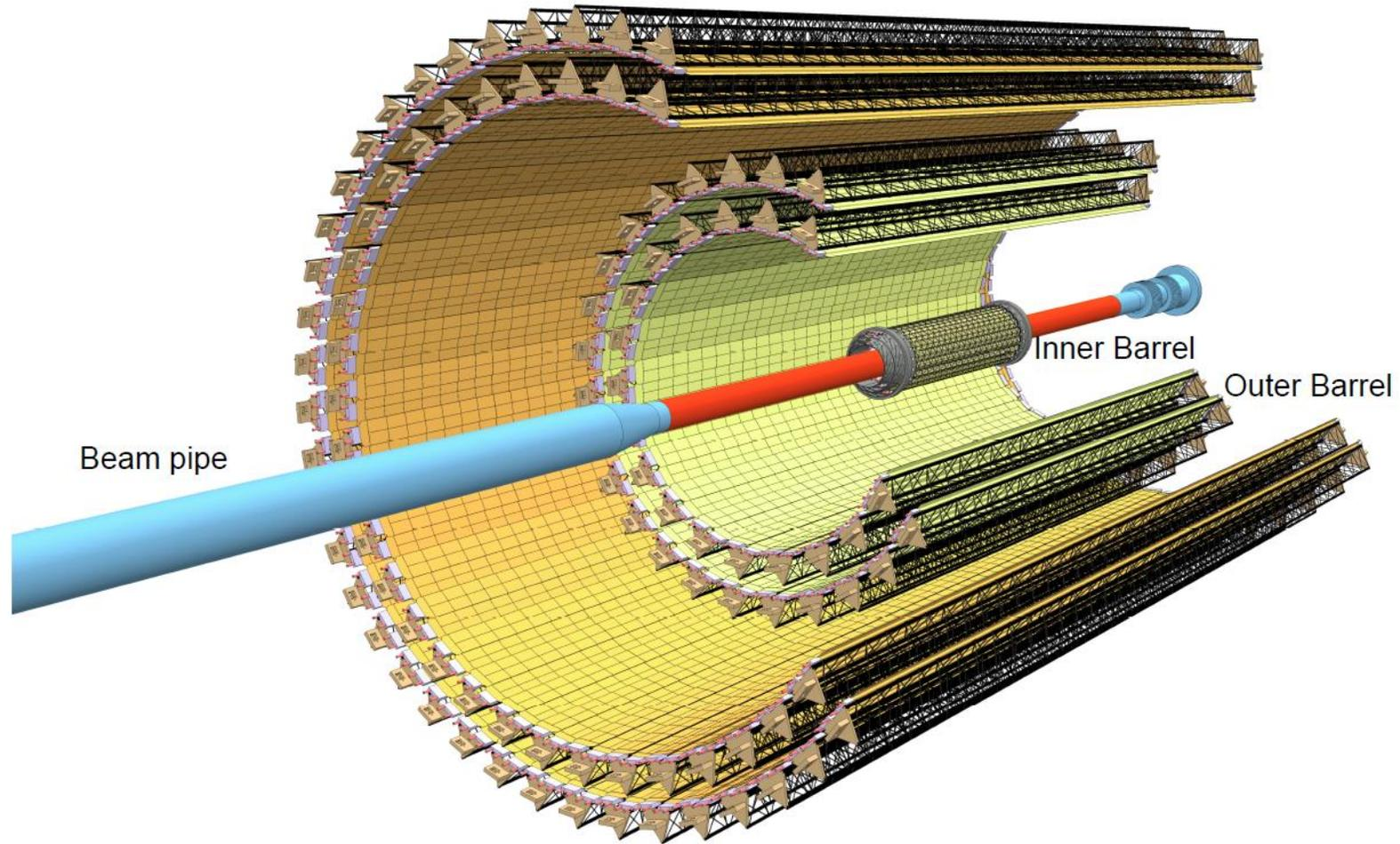
**Figure 1.1:** Layout of the new ITS detector.
