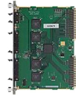
TQDC16 (16-channel time and charge digitizer)
