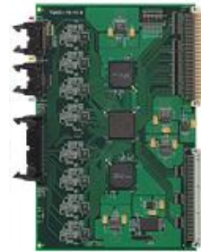
TQDC16 (16-channel time and charge digitizer)
