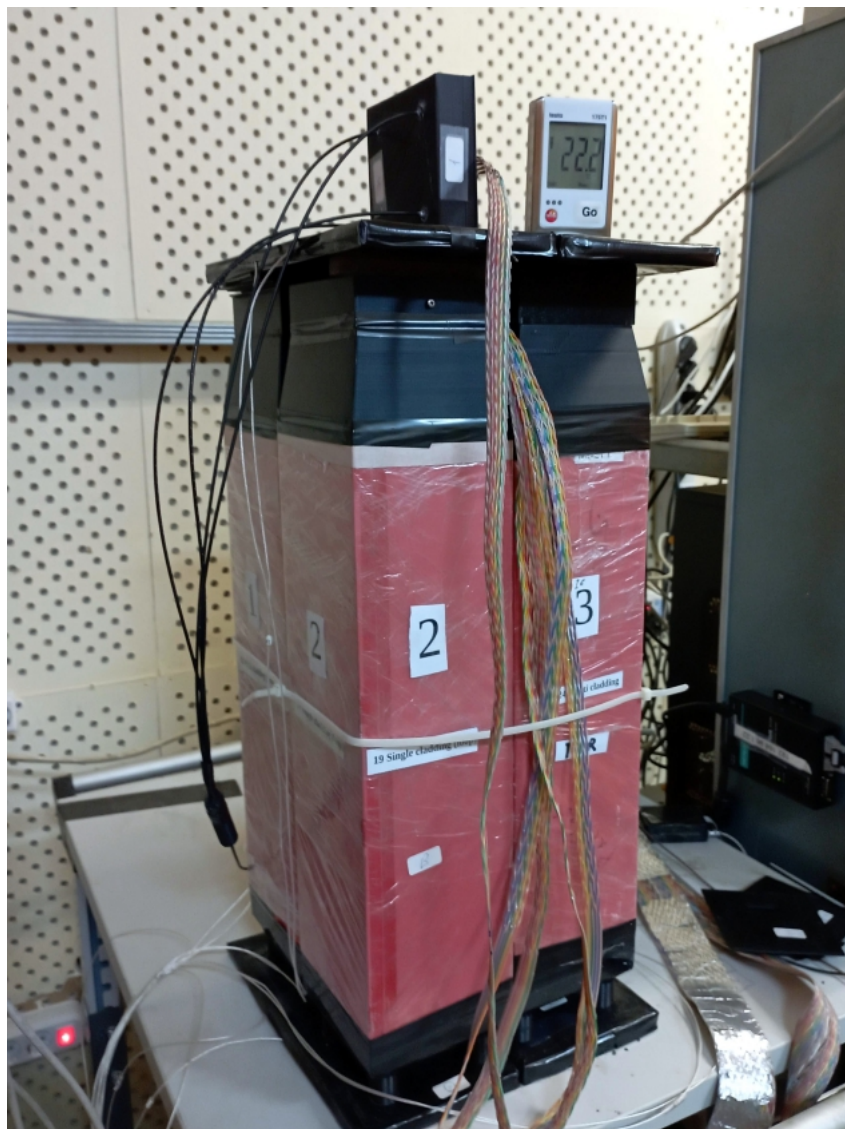
Figure 6.13: Photo of the calorimeter test setup consisting of 4 modules of the size 11 \times 11 \text{ cm}^2 , with the total cross-section of 22 \times 22 \text{ cm}^2 . The environment temperature was measured by thermistors, provided for each of the 4 MPPC boards, and by a digital thermometer as well. One of the boards in light protection cover and the digital thermometer were placed on top of the setup. The optical fibers (visible on this photo) distributed the light from the LED generator.
