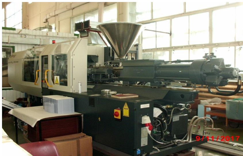
Figure 6.8: Thermo plastic injection molding machine, general view.
