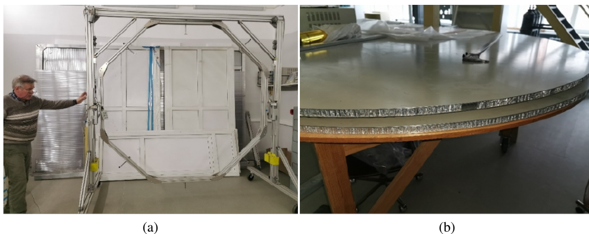
Figure 9.39: (a) Technological equipment for assembly. (b) Octagonal rotary platform and a portable honeycomb board for assembling are shown. The diameter of the portable board is 2300 mm, the thickness is 50 mm.
