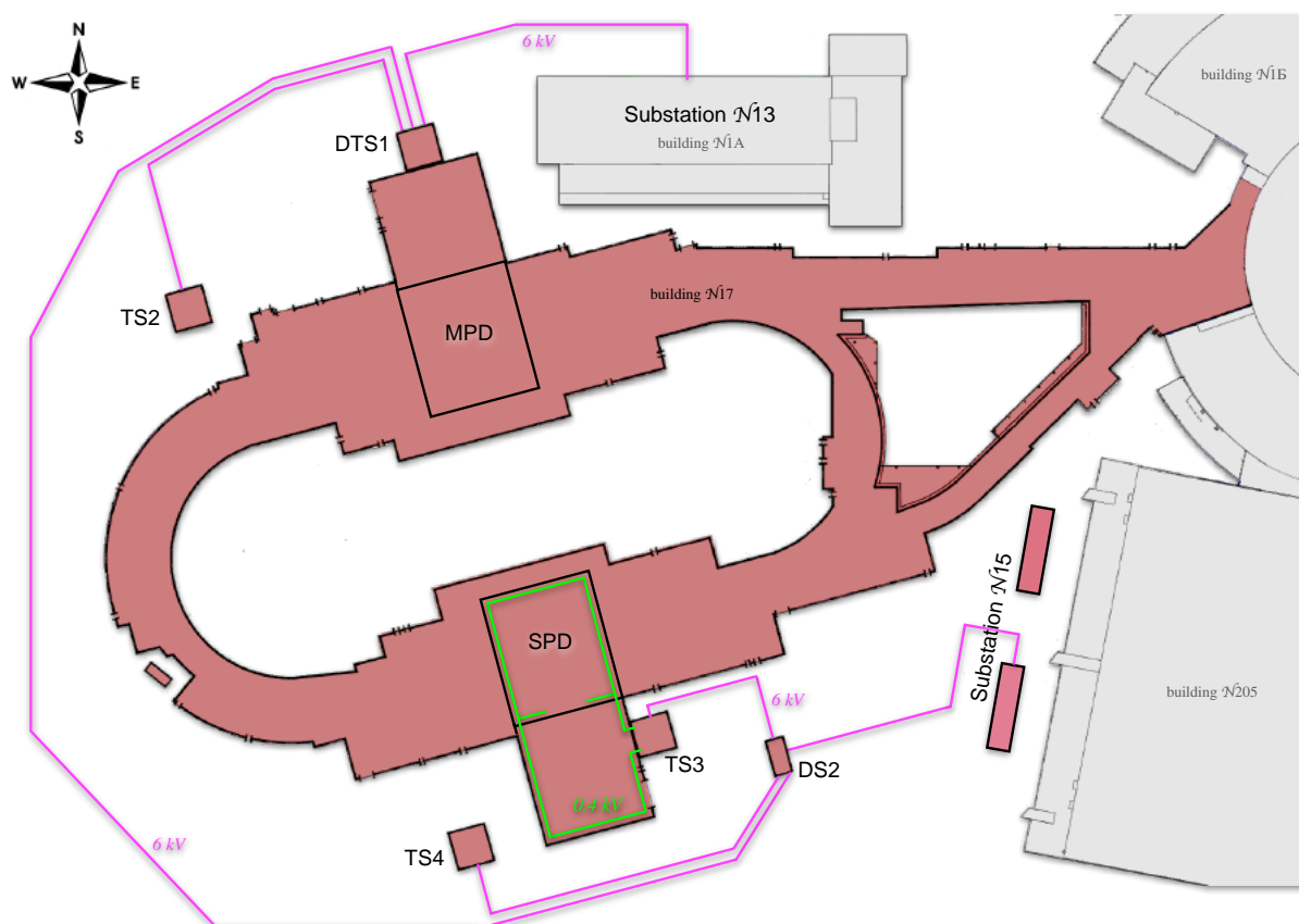
Figure 15.6: Top view of building N17 (the NICA collider) with indications for elements of the SPD power supply system. Power lines with an operating voltage of 6 kV are shown in pink. Power lines with an operating voltage of 0.4 kV are shown in green.
