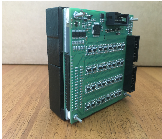
16-channel scintillation detector 2x2x2 cm 3 coupled with 16-channels Hamamatsu S12572-010P SiPM board.
