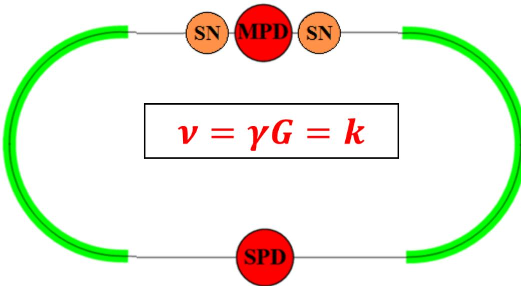
Polarized beam is injected from Nuclotron to the NICA collider at energy which correspond to integer spin resonance
