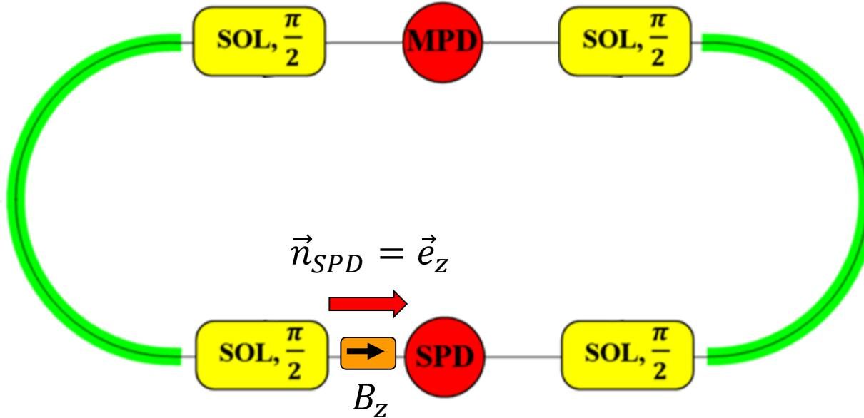
The direction of the stable polarization  $\vec{n}$  coincides with the navigator solenoid axis  $\vec{e}_z$  at the solenoid's location. Outside of the navigator, the direction of  $\vec{n}(z)$  is determined by magnetic fields of the lattice
