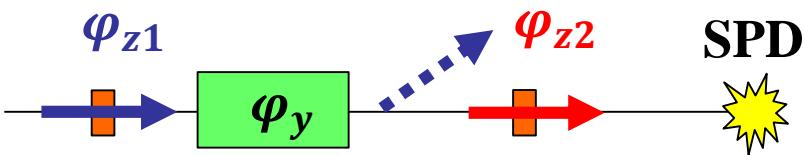
$\varphi_{z1}$  stabilizes the longitudinal polarization before the dipole ( $\varphi_y = \gamma G \alpha_{orb}$ )
