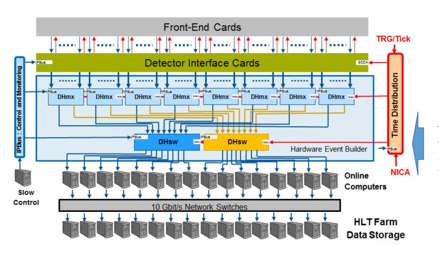
The switches (DHsw) perform the final level of event building and distribute the assembled events to 20 (?) on-line computers.
