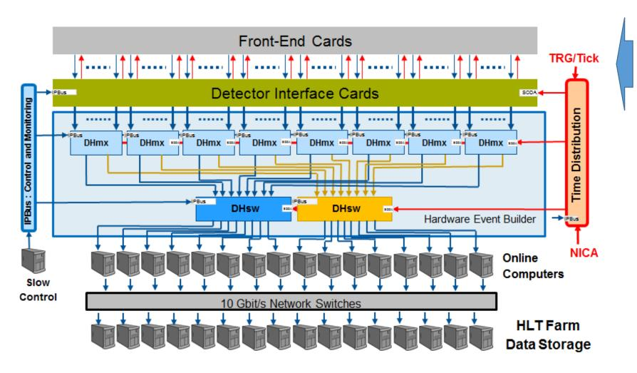
Slow control accesses FEE via the detector interface cards (DIC) using UDP-based IPBus protocol.
