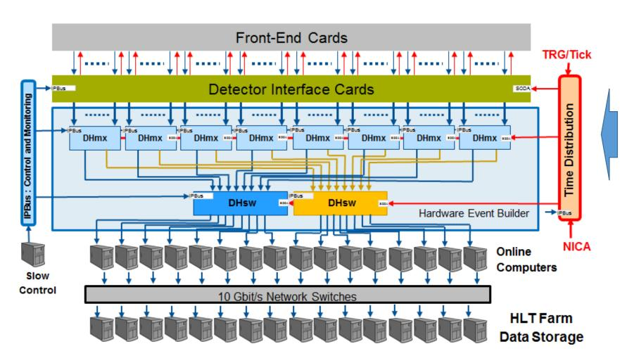
The multiplexer (DHmx) modules receive detector information via serial links, verify consistency of data, and store them in DDR memories.
