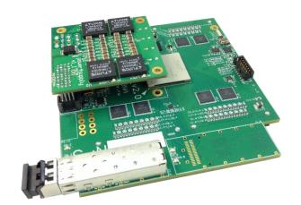
ADC64s2 (designed for MPD) is a 64-channel 12-bit 62.5 MS/s ADC with signal processing core and Ethernet interface. It has dedicated serial links for clock synchronization and data readout. Was it tested in a trigger-less mode?
