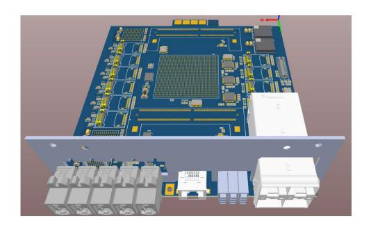
One and the same hardware FPGA-based module developed in TUM can be programmed either as a multiplexer or as a switch.
