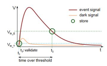
PASTA provides measurement of time and charge of the signal from *microstrip* sensors.
