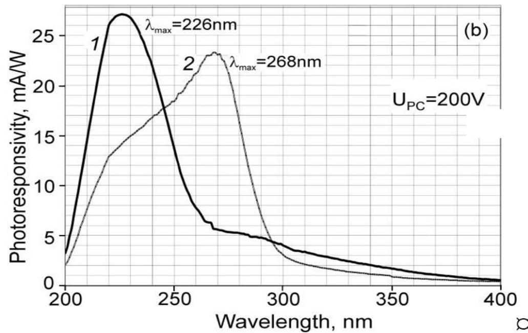
Good spectral range, but high dark noise at level 1 uA. **One need 2-3 more production iterations to eliminate noise and complete this device.**
