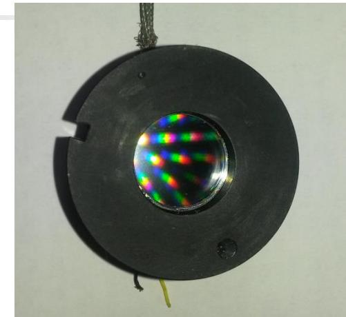
MCP consists of a two-dimensional periodic array of very-small diameter glass capillaries (channels) fused together and sliced in a thin plate. A single incident particle enters a channel and emits an electron from the channel wall.
