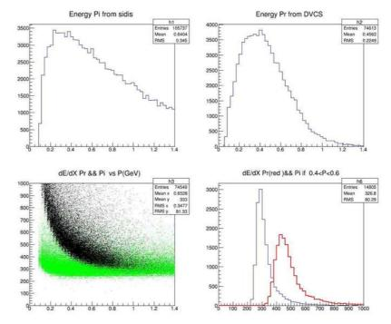
The results for protons (red line) from HepGen (DVCS) and pions from PYTHIA (SIDIS) and thickness of the silicone detector - 0.5 mm
