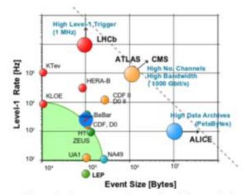
Maximum allowed trigger rate determined by typical event size:
