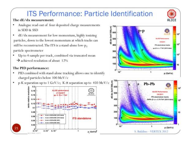
From this analysis it is possible to make the following conclusions: - for this configuration of the detector (3 layers of a silicon) of dE/dx the technique allows to separate pions and protons for the range of momentum lower than 0.5 GeV;
