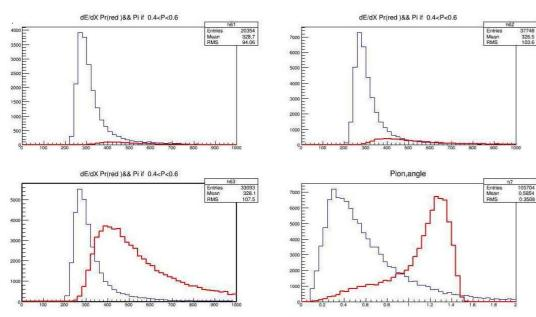
The total energy loss for protons from HepGen (DVCS) and pions from Pythia(SIDIS) and thickness of the silicone detector - 0.3 mm and for three ranges of scattering angles, 0.24-0.36 rad. (the left-hand top schedule), 0.36-0.64 rad. (the right top schedule) and 0.64-1.57 rad. (the left-hand lower schedule). The right lower panel shows the scattering angle
