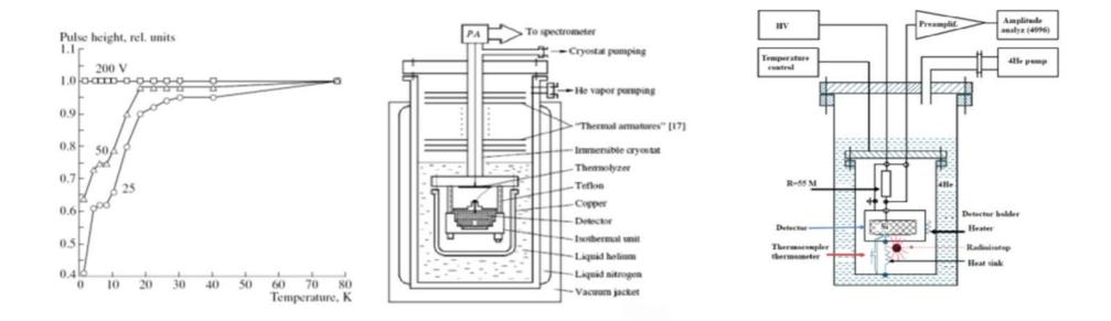
Stable performance of this and other type of detectors at the temperature up to 1K ° requires higher working voltages.
