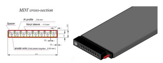
The system of MDT layers with Fe layers called by Range System (RS) is used in SPD as moun detector and main element of Particle Identification System. It can provide the clean (>95%) muon identification for muon momenta grater than 1 GeV. The combination of responses from EM calorimeter and RS can be used for the identification of pions and protons in the wide energy range.
