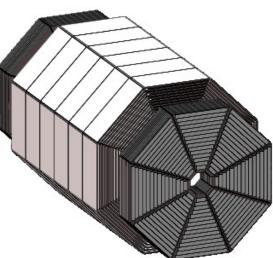
The Range System consists of two parts: Barrel and two End cups.
