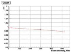
Figure 9. Straw efficiency versus particle rate in a straw.
